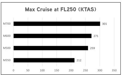
The M700 Fury is up to 20% less expensive to operate per hour than competitors\* and 11% faster than any M-Class before, with a maximum cruise speed of 301 ktas.
